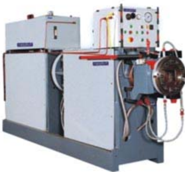
Figura 3.12 – Extrusora RAM industrial 19 .
