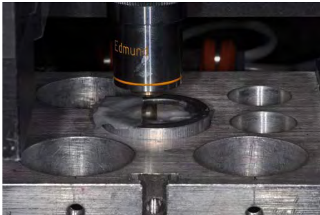
Fig 1 Beams and damp gauzes during the nanoindentation experiment
